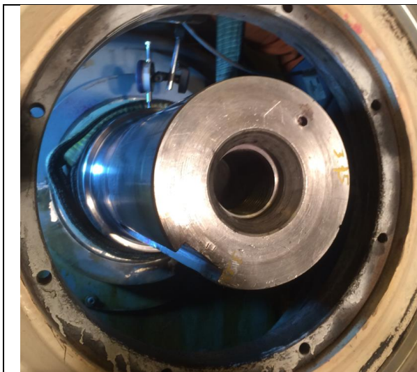
Dial indicator on the shaft seal bushing fit
