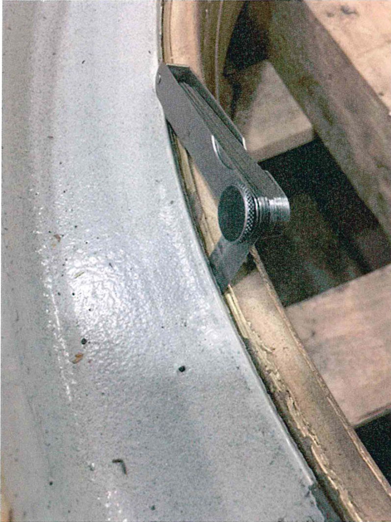
FIGURE 8 - .010" (.25mm) FEELER GAUGE INSERTED BEHIND SEAL
