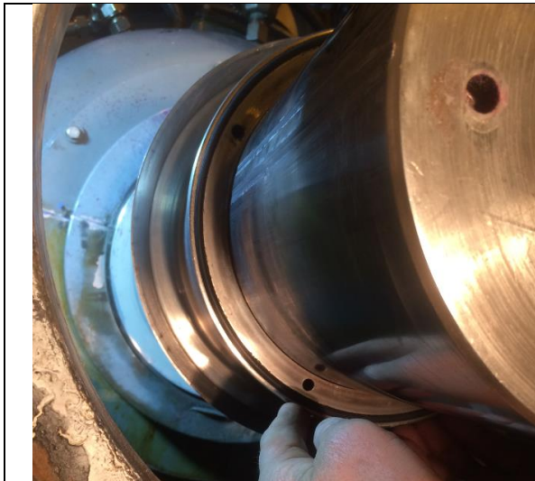
During the installation of the seal bushing
