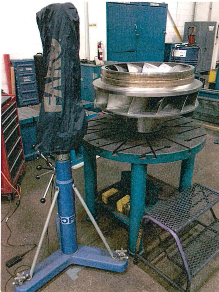
FIGURE 2 – RUNNER SET UP IN FARO ARM WORK STATION
