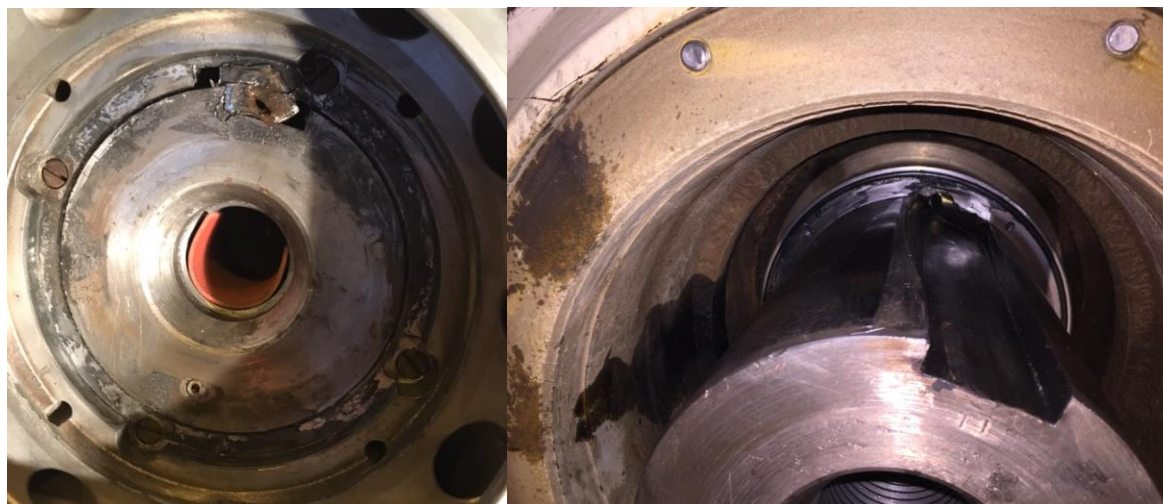
Figure 2 – Rolled Key and Shaft Keyway Damage
