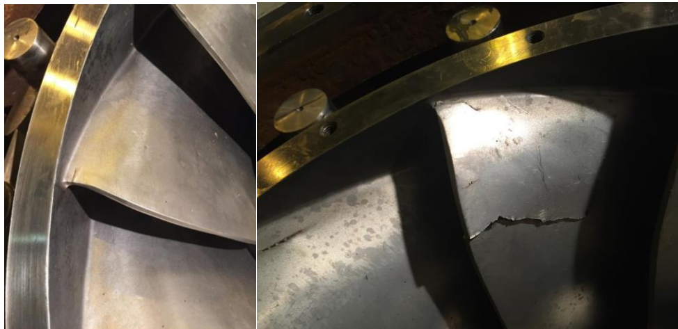
Figure 1 – T1 Turbine Runner Showing Blade Cracks
